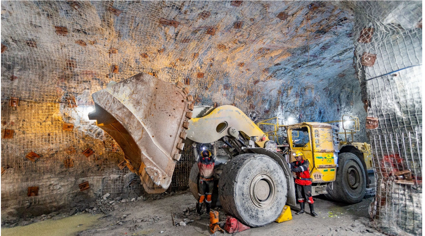
Photo: (L-R) Metsobane Mokoena, Fitter, MRC Engineering and Thabo Makgoba, Foreman, MRC Engineering, conducting maintenance at the 750-metre level workshop on the Ivanplat's Epiroc battery electric 17-tonne Scooptram
