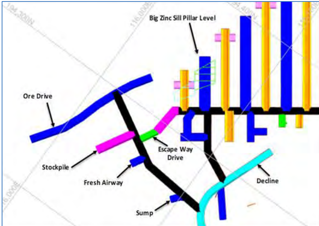
Figure 16.39 Southern Zinc Longitudinal Open Stopping Level Layout
