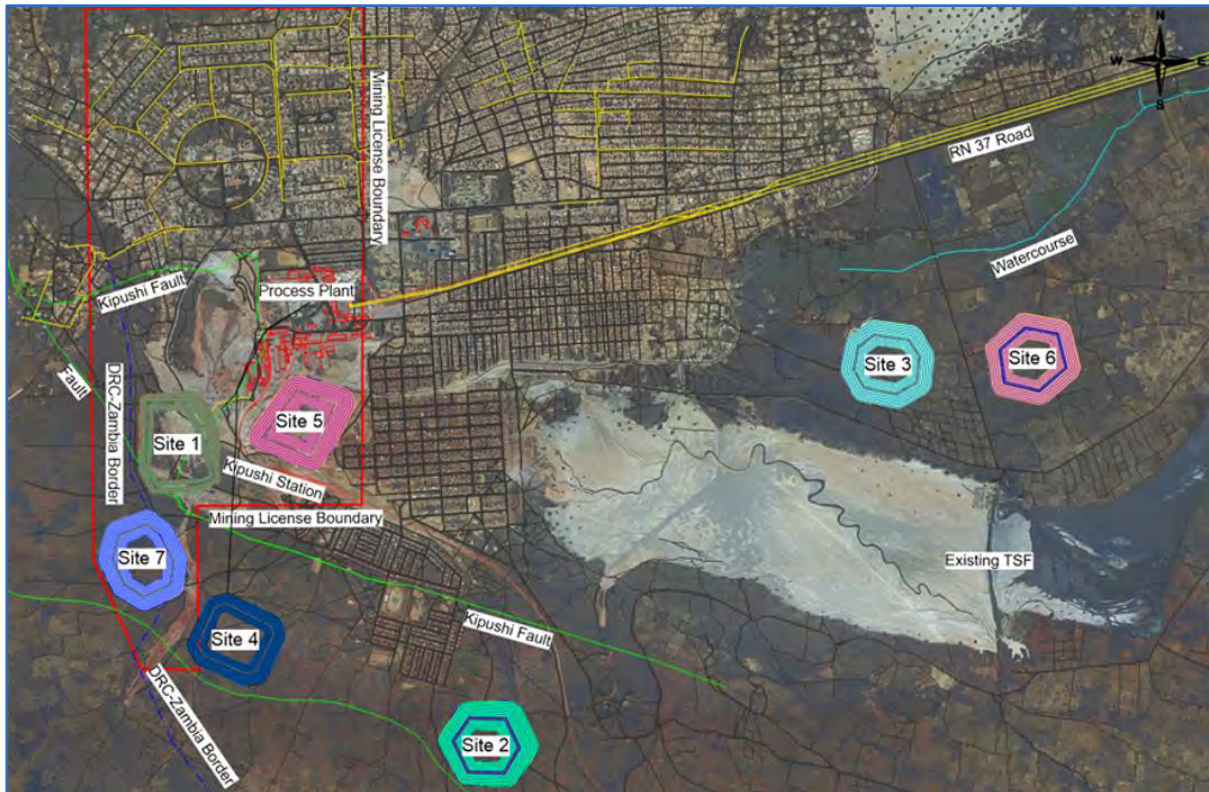
Figure 1.5 FS Tailings Dam Locations – Site 4 Selected for the Study
