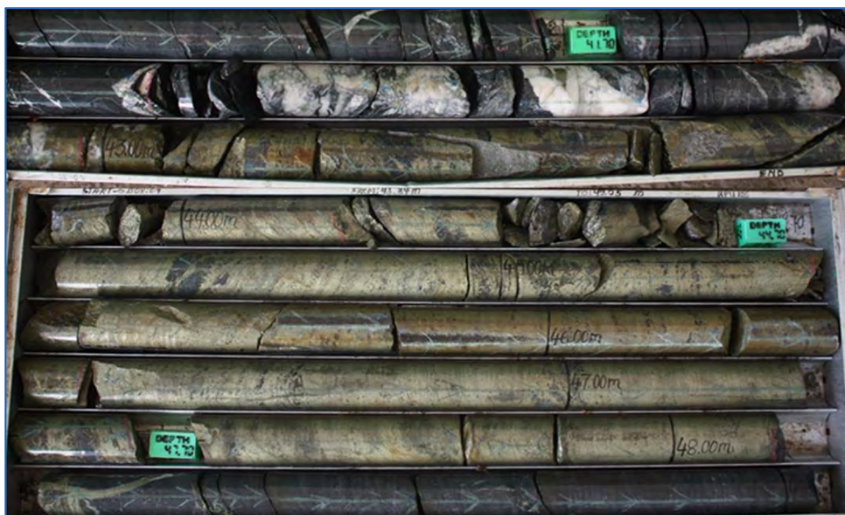
Figure 7.22 Drillhole KPU105 Showing Massive Chalcopyrite Mineralisation in the Upper Kakontwe near the Northern Limit of the Fault Zone
