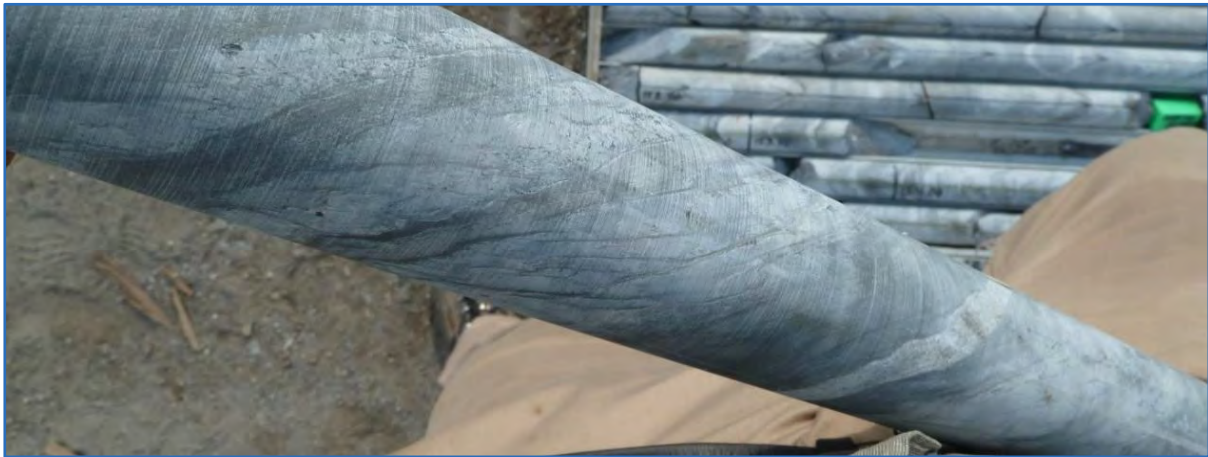
Figure 7.6 Interbedded Dolomite-Shale/Siltstone Unit in the Upper Kakontwe Formation at 153 m in KPU070 (hole orientation –35 to 125)
