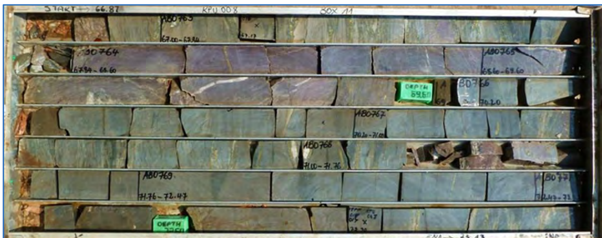
Figure 7.24 Typical Colour Variation in the Série Récurrente Between Dolomite (Purple) and Siltstone (Green)
