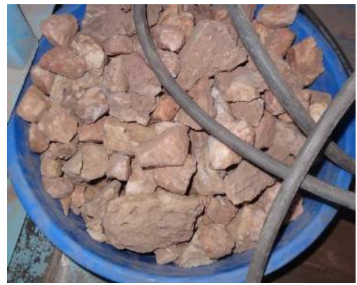
D Coarse quartz blank material used for flushing between samples
