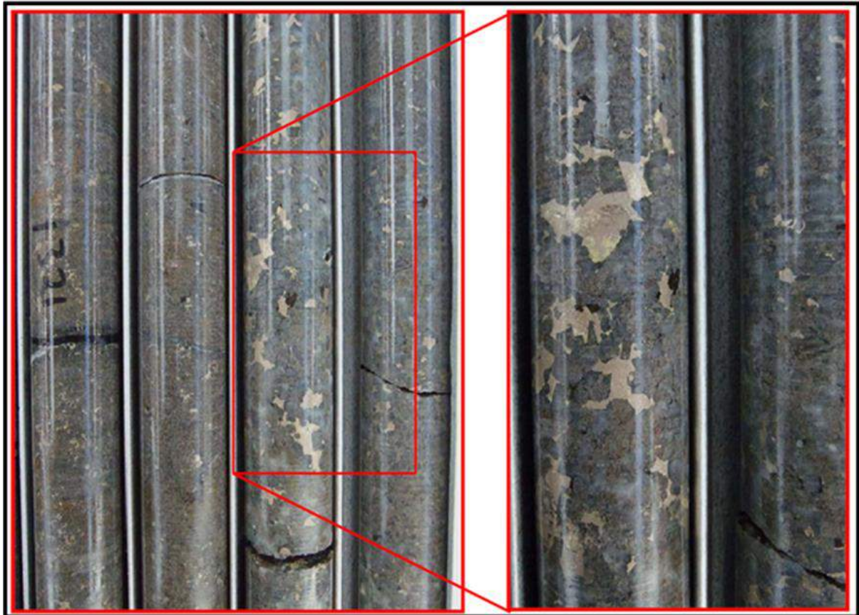
Figure 7.18 Core Photograph from UMT083 at 1,323 m Depth, Illustrating Sulphide Mineralisation
